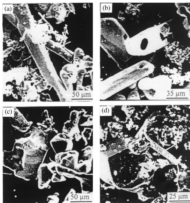
Fig. 5. SEM images of \text{Ag}_2\text{Se} synthesized with \text{Ag}_2\text{CO}_3/\text{Se} = 1.2.5 (a), 1:2 (b) and 1:1 (c) in \text{H}_2\text{O} at 190^\circ\text{C} for 36 h.
